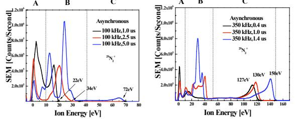
The 'A' ion energy region corresponds to the negative pulse period (sputtering period). The 'B' ion energy region is the energy gained from the potential in the oscillating reverse positive pulse period. The 'C' ion energy region is the kinetic energy gained from the fast and high positive voltage overshoot at the beginning of the positive pulse period
